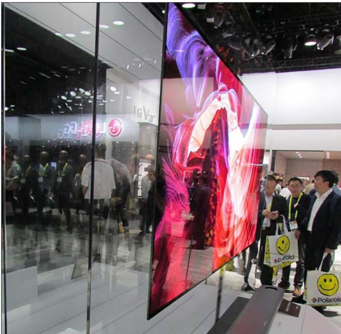
OLED 4K Display: Notice the thickness of glass sheet on the edge, ~0.3inch! (Image Rights: Electronics Cooling®)
