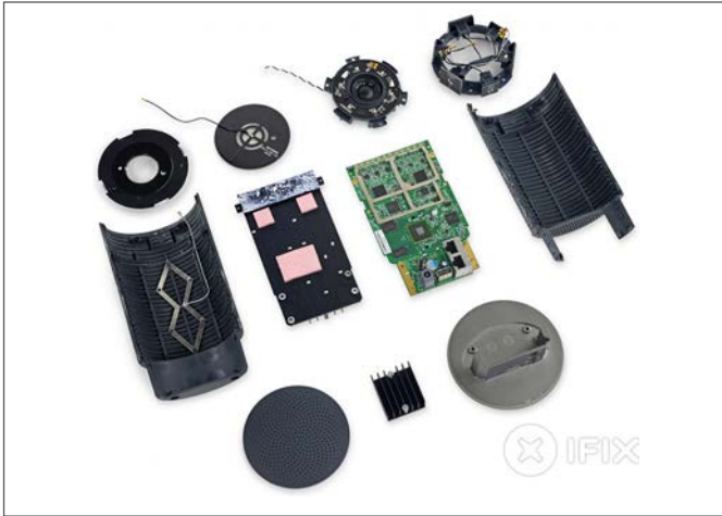
Figure 6. Final tally of components: two heatsinks, cooling-capable cover and most importantly a software-enabled dynamic thermal management environment (not shown!)
