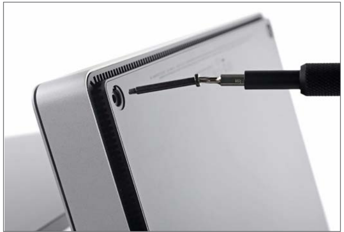
Peripheral Vents for forced air cooling of Microsoft Surface (Image from iFixit)
