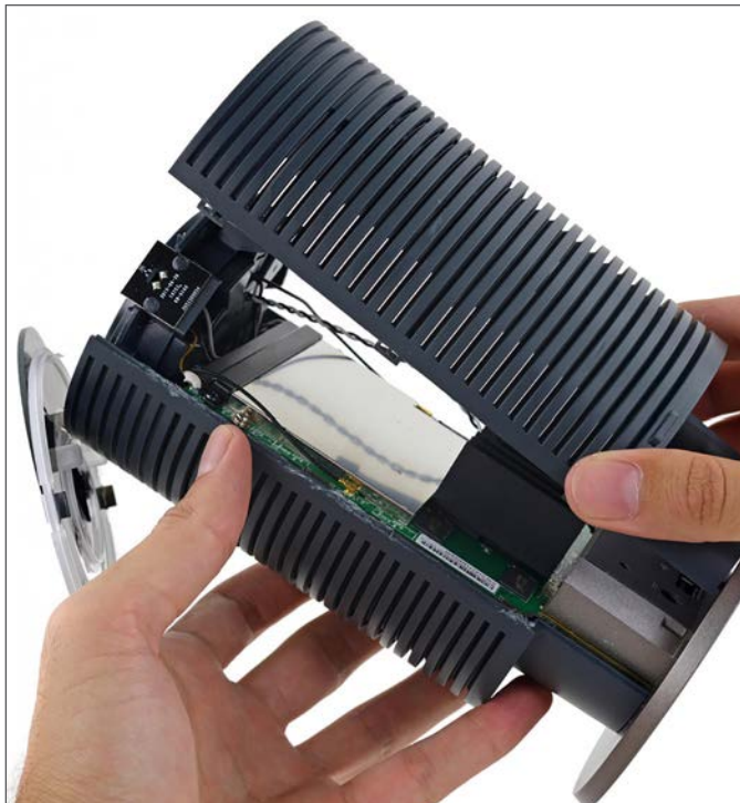
Figure 2. OnHub with the inner cover removed.
