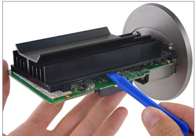
Figure 4. Larger heat sink contacting multiple components.
