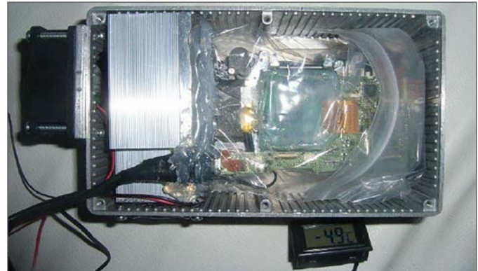
Re-purposed Canon 450D (XSi) with Peltier cooling assembly for astronomy imaging (source)
