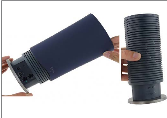
Figure 1. OnHub with the cover removed. The IoT Hub is passively cooled with slits for air circulation
