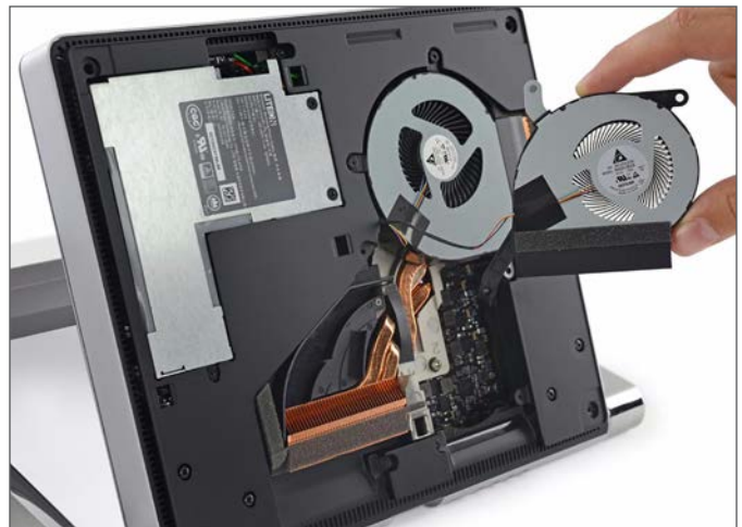
DC Brushless motor-based fans for forced air cooling of Microsoft Surface (Image from iFixit)
