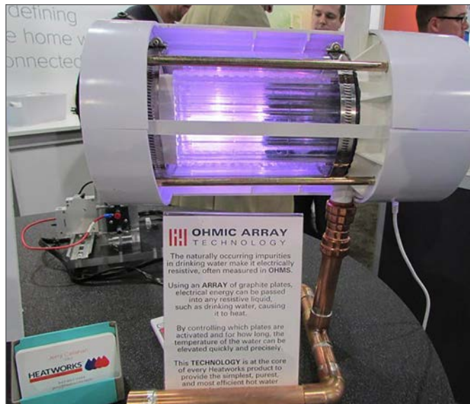
Ohmic Array Water Heater (Image Rights: Electronics Cooling®)
