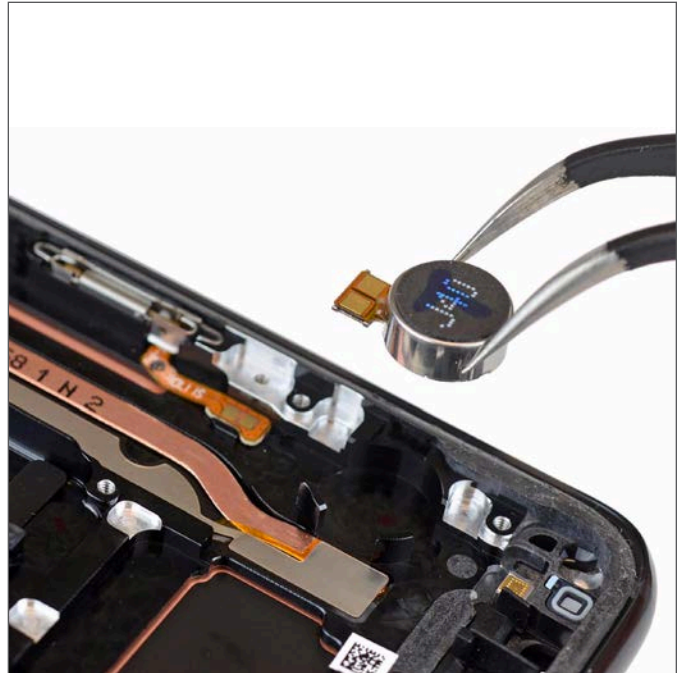
Heat pipe carrying the heat away from processor to the handset's mid-plane (Image from iFixit)
