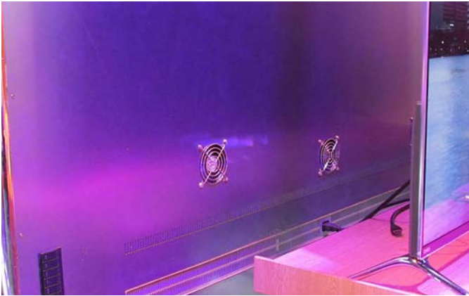
120inch 4K/8K UHD Display: Back Side Showing Cooling Fans (Image Rights: Electronics Cooling®)
