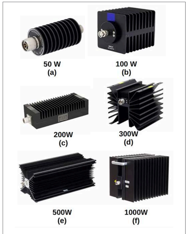
Figure 6: A sampling of attenuator and termination heat sink topologies with varying power handling. The (a) annular fin heat sinks are often used on attenuators up to 50 W while parallel plate attenuators can be used for higher power handling attenuators such as (b) 100W, (c) 200W, and (f) 1000W. Flared fin heat sink designs (d)(e) are often employed for improved natural convection cooling over parallel plate heatsinks.
